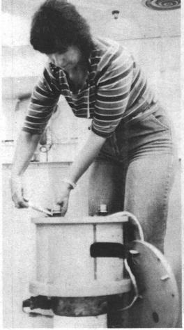
MARILYN HIGLEY disassembles the centrifuge test equipment for the B61.
